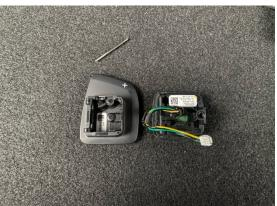
Now take the new paddle and place it in the shifter paddle bracket, be careful to install the small silicon spring correctly. Then use force to push the aluminium pin back into place in the correct orientation.
