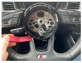
Make sure to unplug the electrical connectors to the paddles on both sides!
